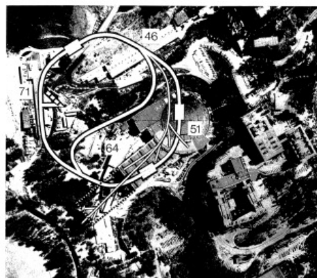
Aerial view of the Berkeley site with the location of the proposed relativistic heavy ion machine superimposed. The numbered buildings refer to existing facilities which could be used with the new machine.
