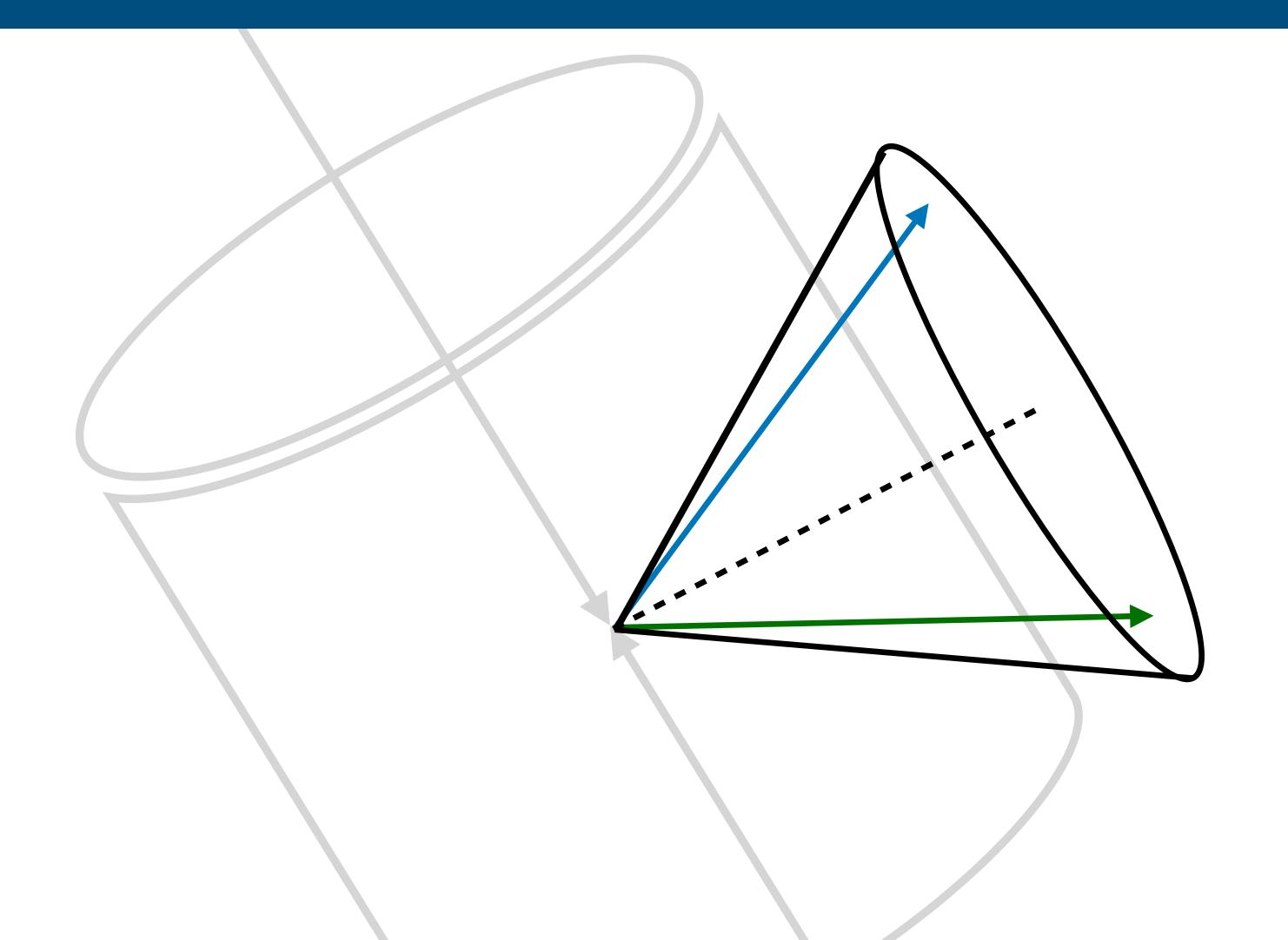
Rotate reference frame so jet axis lies along z axis
