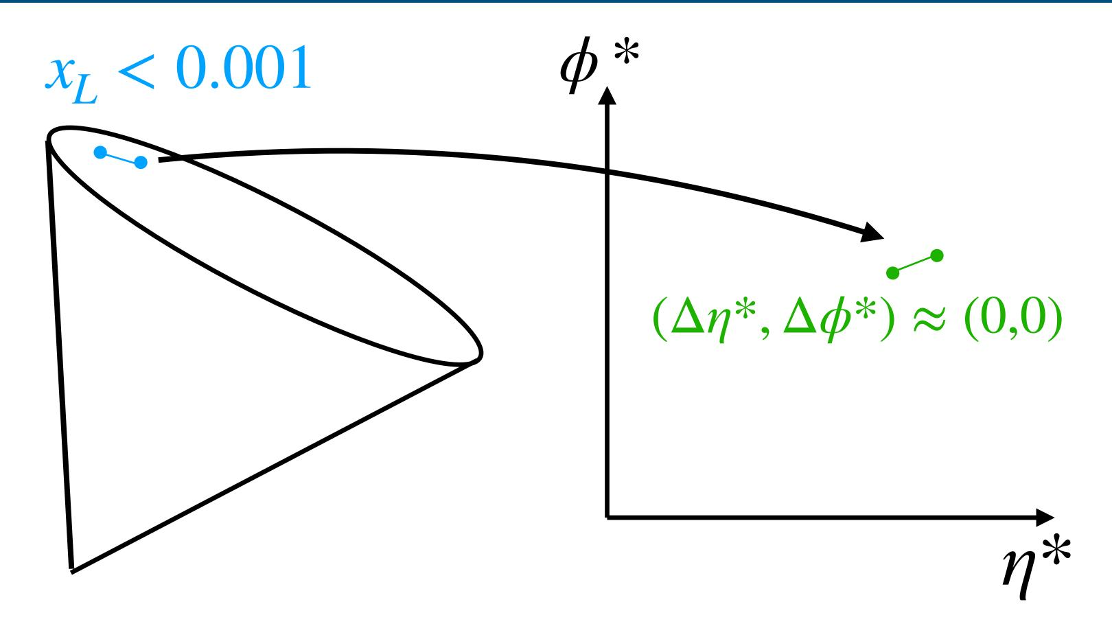
Particles close to each other in lab frame are also close to each other in jet coordinates
