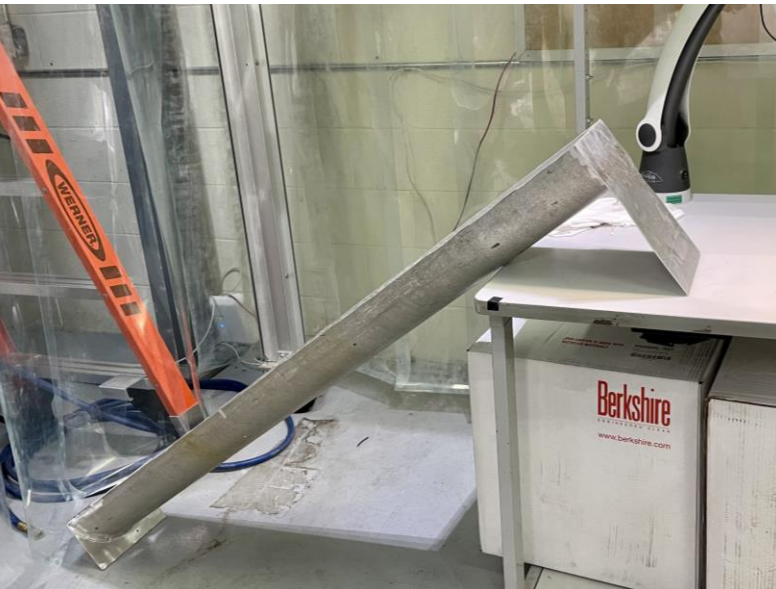
Bar end immersed in acetone bath
