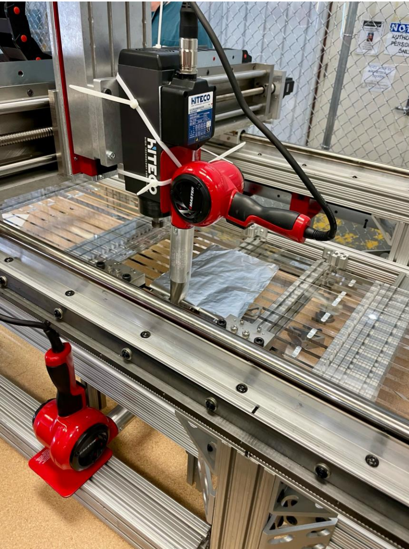
Heat guns softening glue joints between bars
