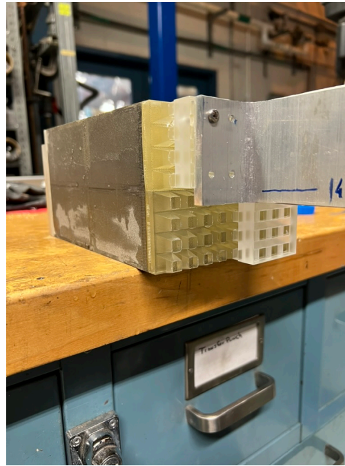
Removal of SiPM boards No damages to LG
