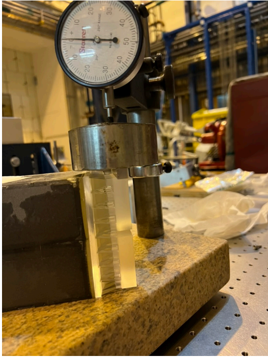
Long term shear test ~ 6 months, no issues.
