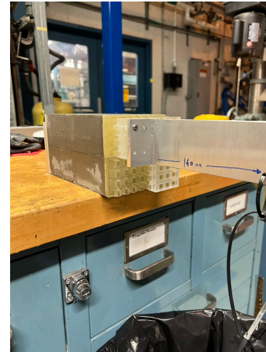
Static peel tests, Safety factor ~ 100
