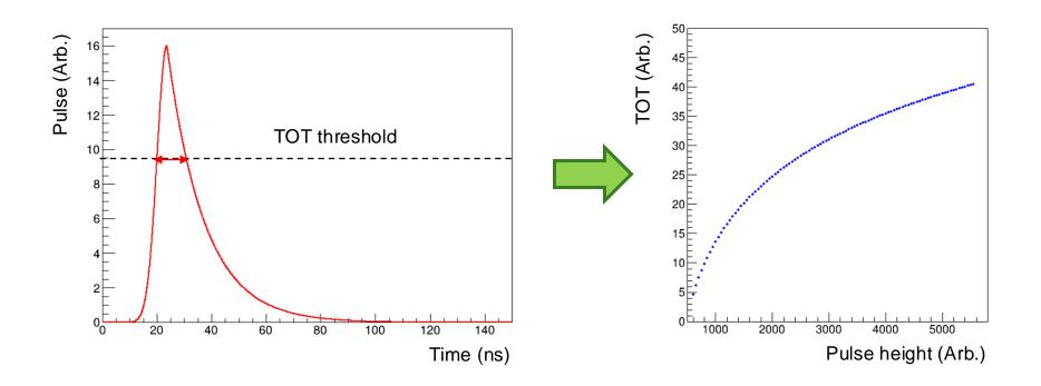
• The TOT value can be 1 vs. 1 matched to the pulse height, thereby the pulse height can be reconstructed precisely.
