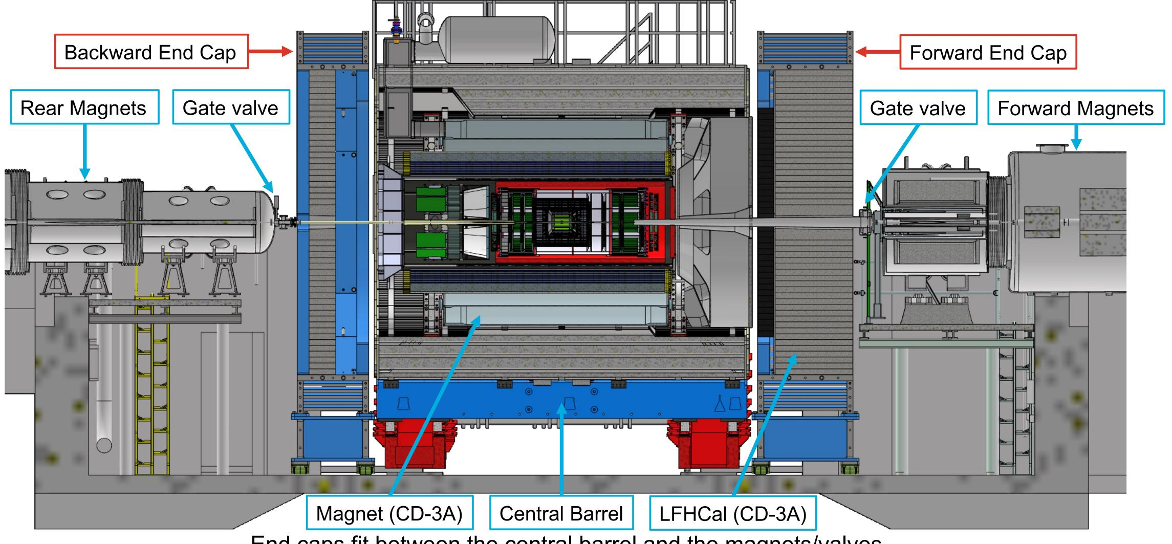
End caps fit between the central barrel and the magnets/valves
