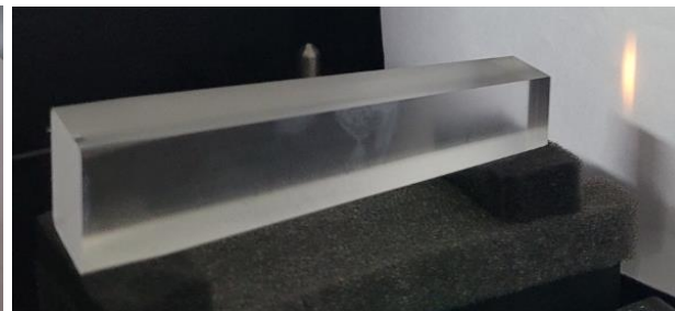
Different beam spread for one-side polished (#3)
