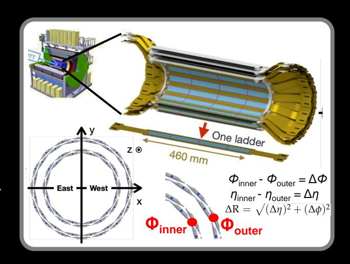
The 2-layed INTT is used for tracklet reconstruction to measure  $dN_{ch}/d\eta$
