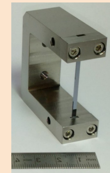
Bent silicon crystal developed for CERN LHC beam collimation
