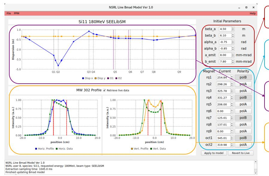
Initial beam parameters used by model
