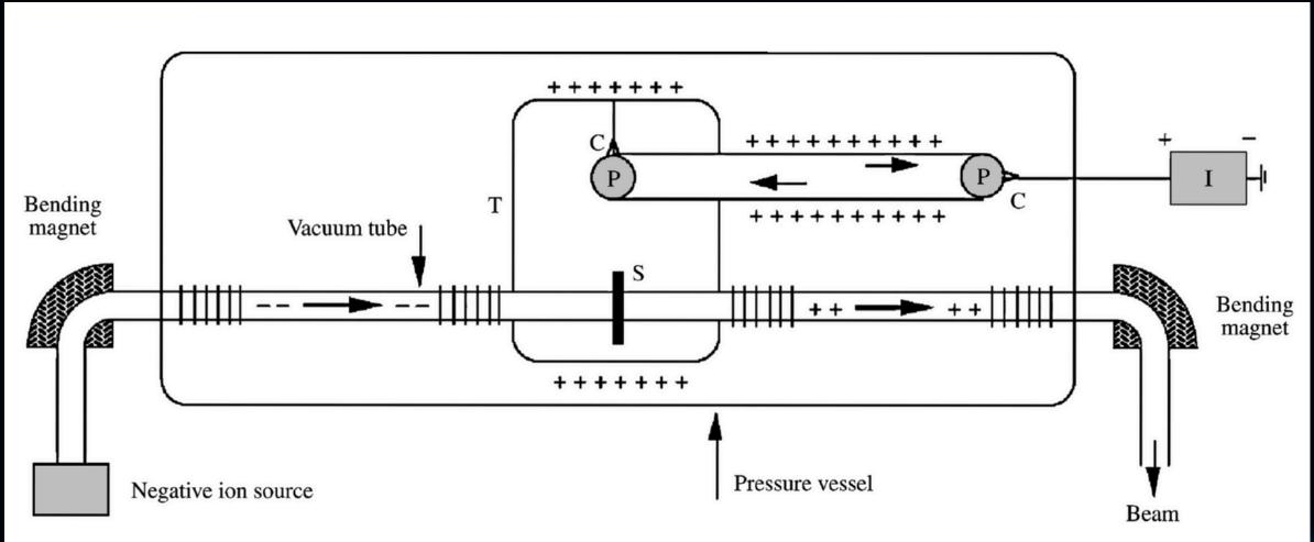
Figure 4.1 Principle of the tandem van de Graaff accelerator
