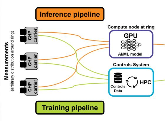
An Edge AI/ML model will have the potential to interact with the machine in streaming mode without waiting for a response from the controls system, but event synchronization may be necessary.
