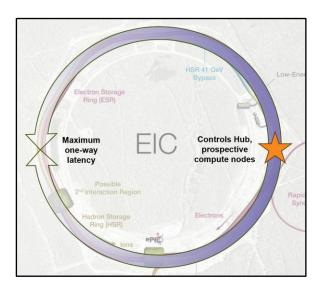
For an Edge Al/ML application to be deemed feasible, the entire pipeline must be completed within the window dictated by any synchronized event(s). Latencies will depend on compute node location(s), so the consequences of infrastructure decisions on future potential use cases must be well understood. This is a focus of current work. Compute latencies must then be added to this.
