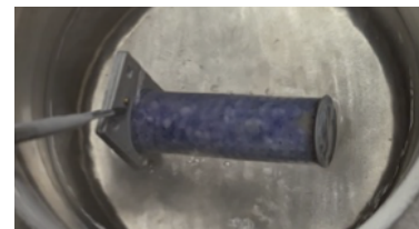
Sample container filled with \text{ND}_3
