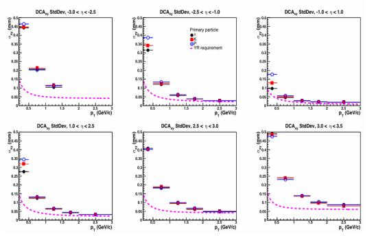
Derived track pointing resolution in the xy plane does not fully meet YR requirements, especially at low p<sub>⊤</sub> and high rapidity
