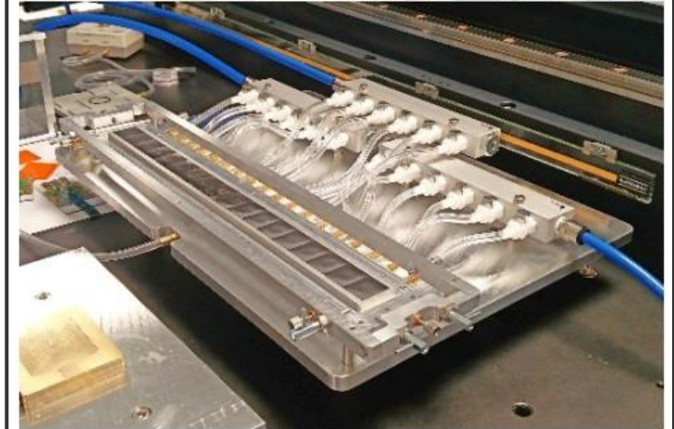
Figure 7.21: Robotic gantry (upper figure) for placement of 17 or 18 MuPIX chips on the vacuum jig (lower figure).
