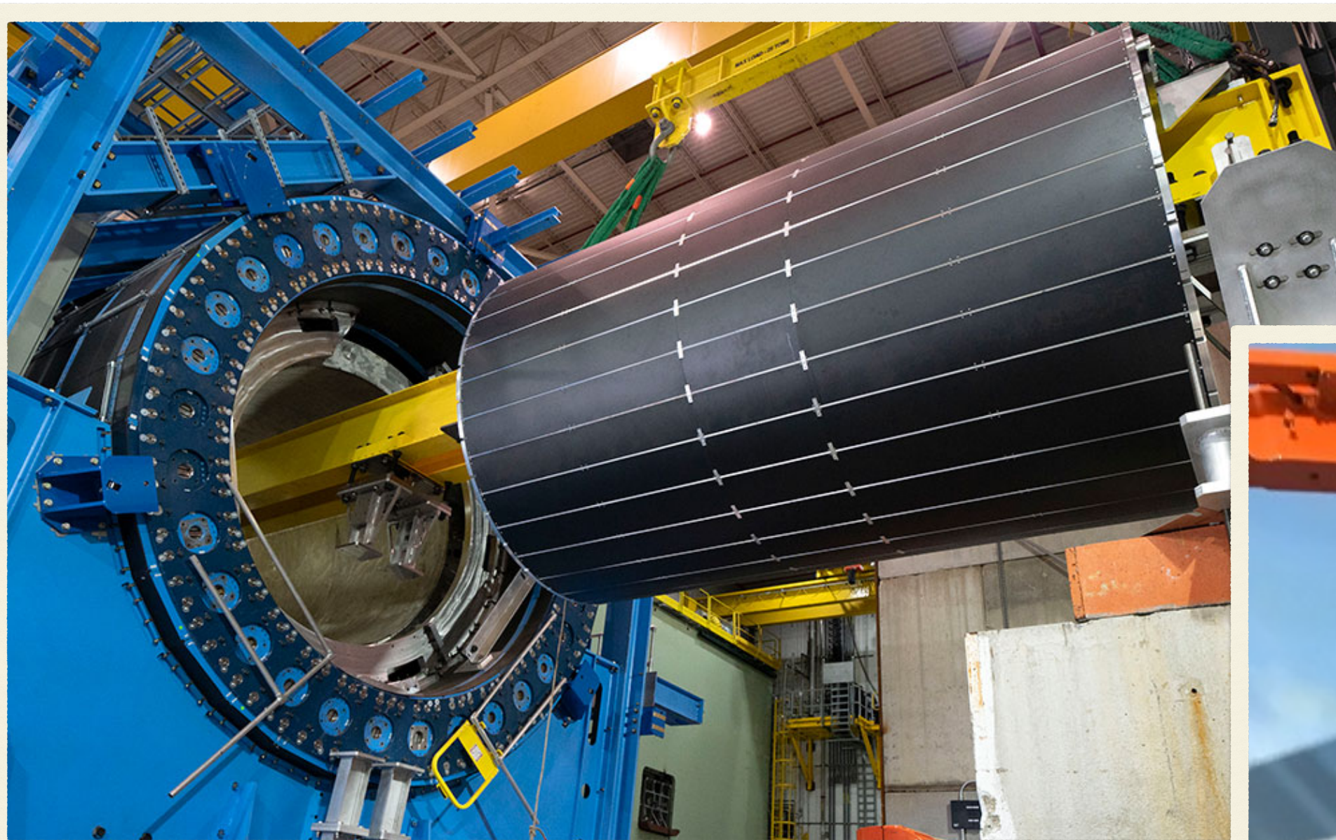
Full iHCal barrel insertion, June 2022
