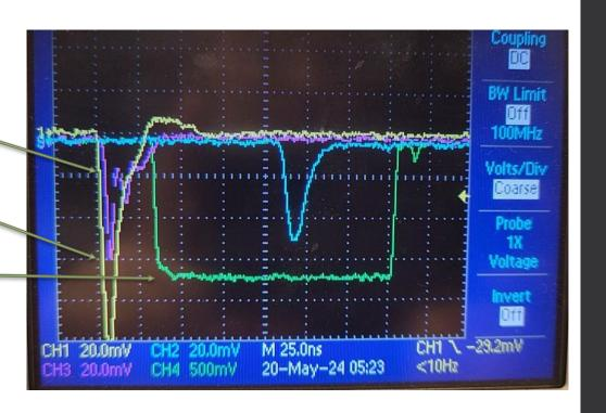
• Delayed (by purpose) signal from SiPM-on-tile
