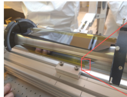
Extra tape was not sufficient: fracture was the source of the successive break in the picture
