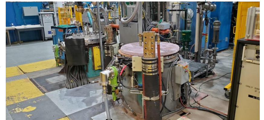
Magnet in Test Dewar and Field Measurement Probe
