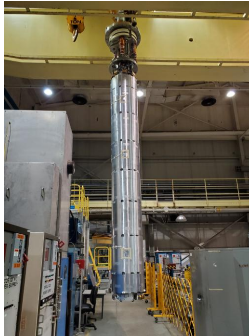
Ready with all power and instrumentation connection-transported to test Dewar
