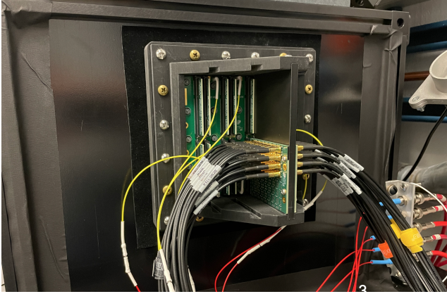
Figure 3. HRPPD #16 mounted on a dark box side wall. One can also see the interface board with a pair of plugin MCX adapters.
