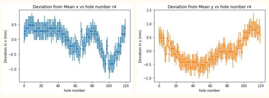
The error in determining the hole center is estimated to be +/- 3 pixels, this converts to about +/- 0.3 mm
