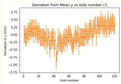
The error in determining the hole center is estimated to be +/- 3 pixels, this converts to about +/- 0.3 mm
