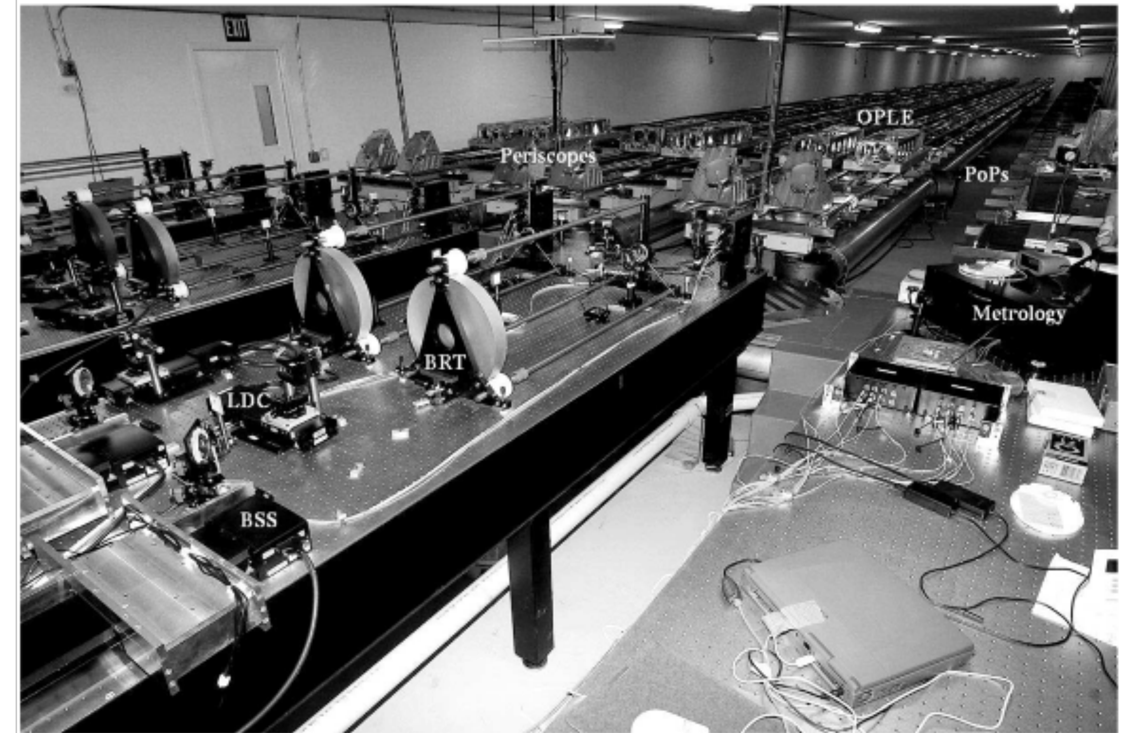
Beam line path length control at CHARA
