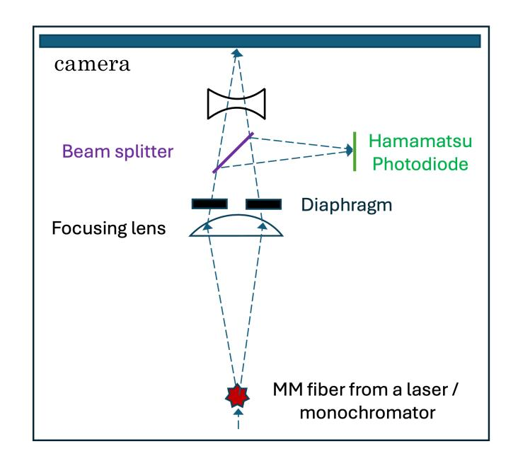
Using a combination of a convex lens and concave lens, the beam spot can be enlarged by a factor of 2, while keep uniform profile.
