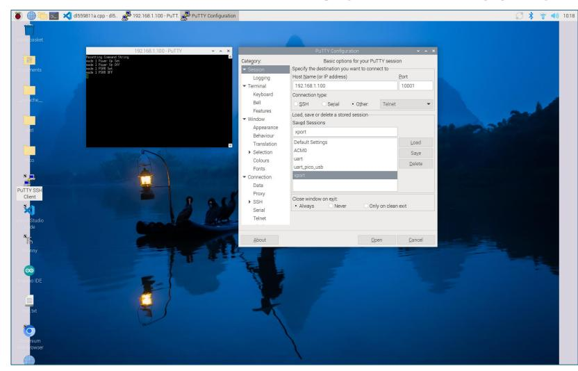
Opening a PuTTY Telnet Session gives you access to The command line interface of the control board.
