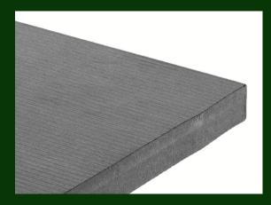
Metapor aluminum is porous to let air and moisture escape, which prevents bubbles and blemishes. These sheets must be milled to expose the pores; average pore diameter is 0.0006" with a total porosity of 15%.
