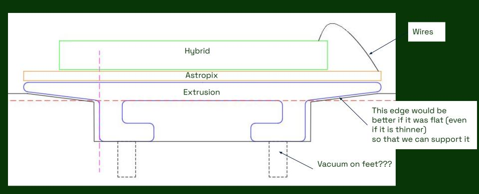
The angled edges on the extrusion are highly likely to cause wirebonding problems due to lack of support. A narrow (<5mm) vacuum pedestal in the center will not hold them well enough to prevent tipping.
