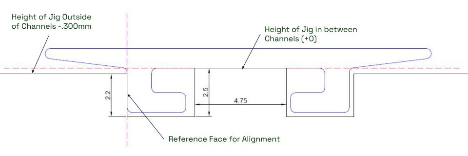
Width in between the channels for vacuum is now less than 5mm. Extrusion may tip. Radiused corner on extrusion means that the reference face is no longer plumb, so central section of jig needs to be 300um higher than the rest (i.e. most of the jig gets planed by 300um).
