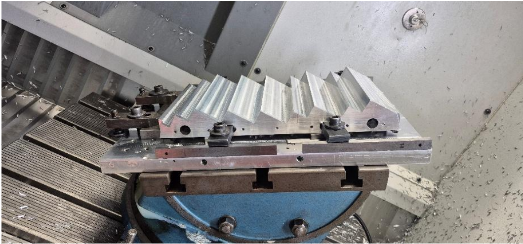
Machining of the steps Metrology testing of the shape < 0,025 mm
