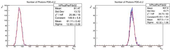
Detector shows Gaussian-like response with relative resolution  $\mu_N/\sigma_N$ =16% for 1 GeV beam and 5% for 10 GeV beam.
