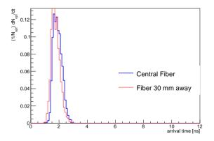
Light propagation smearing is fully included in  $\pm 1$  ns time window.
