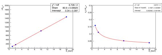
Simulation shows perfect linearity and typical dependence of relative resolution as a function of photon energy:
