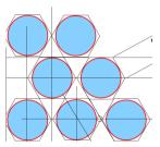
Remark: Twice the larger fibre radius was used for the above images with an effective fibre fraction of 64%; possibly, the final optimal fraction will be about 35%.
