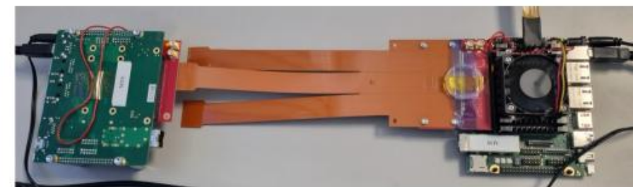
ITS3 FPC test setup and interconnections
