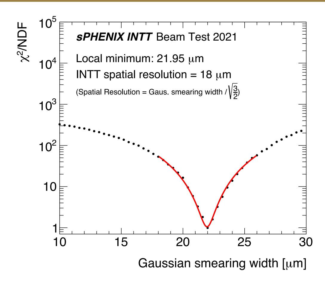
Best matched Gaussian width (local minimum) =  $\frac{3}{2}\sigma_{\text{Ladder}}^2 \rightarrow \text{INTT}$  spatial resolution of 18 µm is observed using beam test data
