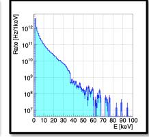
Spectrum of SR photons (> 1 KeV) hitting the inner surface of the IP6 beam pipe. (Jan 2025)
