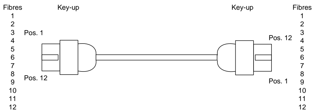
Figure 8 — Multi-fibre connector assembly method type B.
