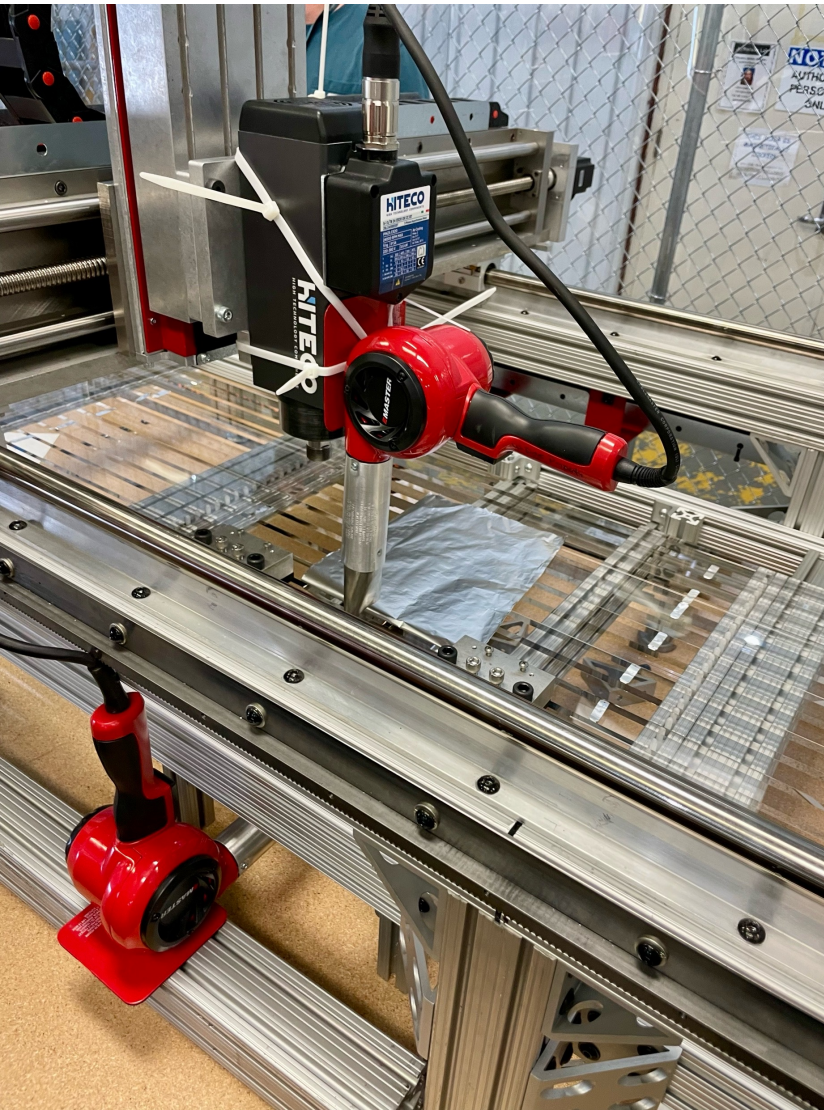
Heat guns softening glue joints between bars
