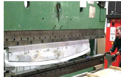
R&D L-bend chamber extrusions received and bent. Demo welds made.
