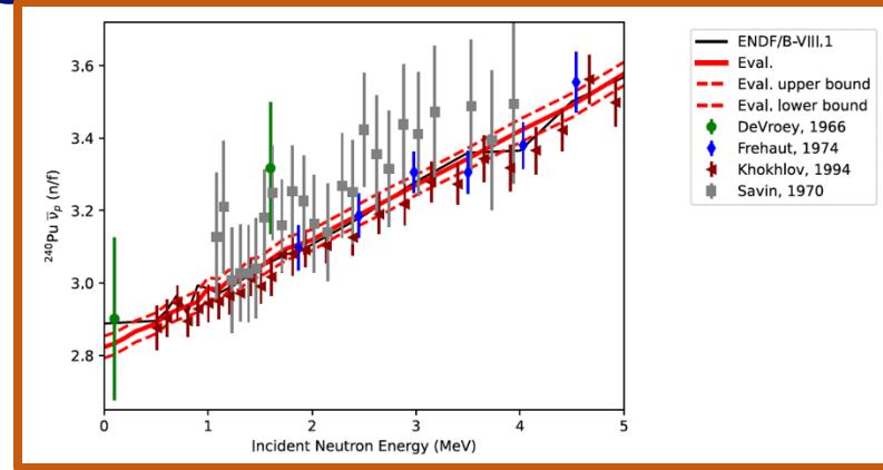
Unpublished DANCE data are being used to guide the evaluation. Experimental data sets from LANL LDRD can be leveraged for robust UQ. Covariances are being developed.
