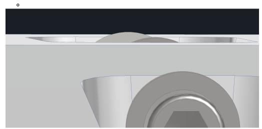
While looking at the model today we noticed that the bolts that connect the sectors were longer than the pockets that they have to fit into.
