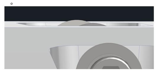
• While looking at the model today we noticed that the bolts that connect the sectors were longer than the pockets that they have to fit into.
