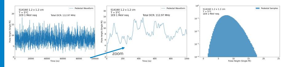
Example simulated baseline and pedestal for S14160 SiPMs at 5 °C irradiated 1e+09 1-MeV neutron equivalent dose
