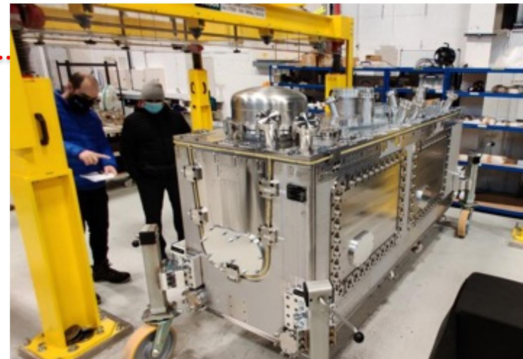
HL-LHC cryomodule at Daresbury Laboratory
