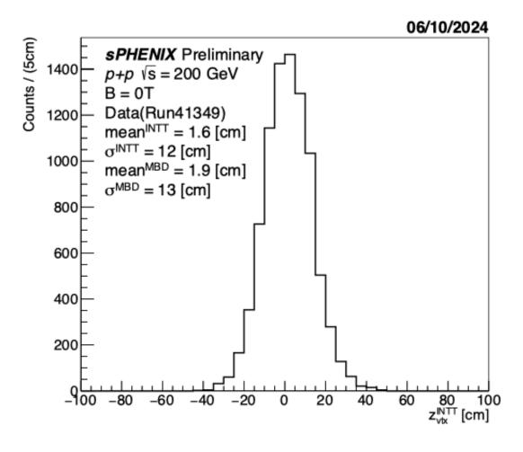
NTT-determined <u>vertex</u> (triggered, field off)
