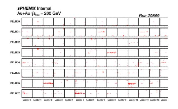
Figure 6: The map of hot channels of run 20869.
