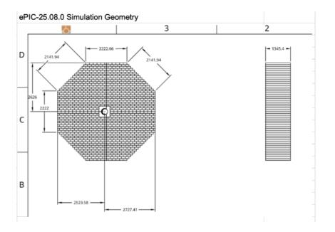
Total horizontal and vertical extent is 2626x2=5,252 mm (25.08 is shorter by 1mm horizontally in simulation)
