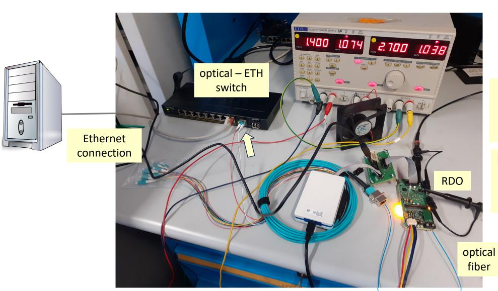
We are currently using this setup to test the US+ / ATtiny I2C communication
