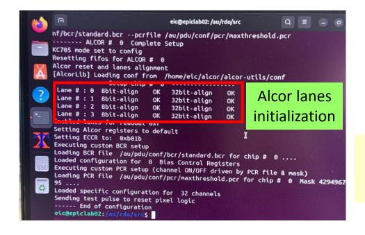
The first RDO setup is mainly devoted to test the communication between the US+ and the Alcor chips
