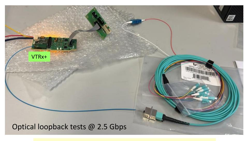
We used the IBERT core on the US+ firmware to test the FPGA-VTRx+ devices on loopback mode @ 2.5 Gbps: no errors found
