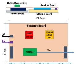
LpGBT: 10Gbps Rad Hard Transceiver ASIC VTRX+: Rad Hard 4xTx (10Gbps) + 1Rx (2.56Gbps) MUX64: Rad Hard 64-channel analog multiplexor
