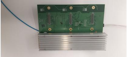
Cooling fins above act as the detector's "Cooling Manifold" (slide 2)
