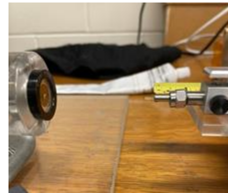
Optical grease at contact
