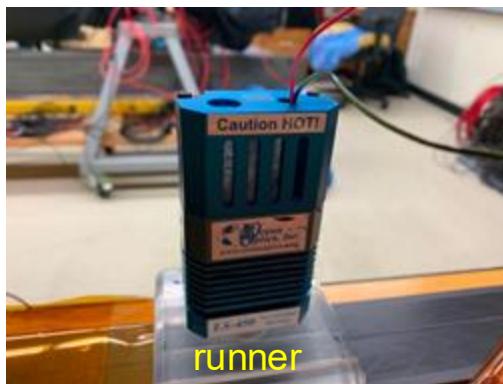
LED 370 nm; slides on acrylic runner
