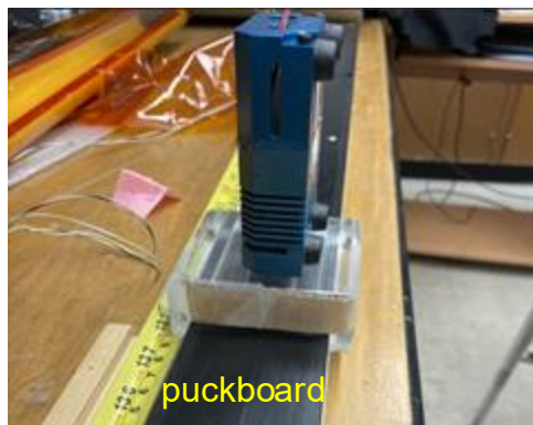
LED 370 nm; moves along puckboard
