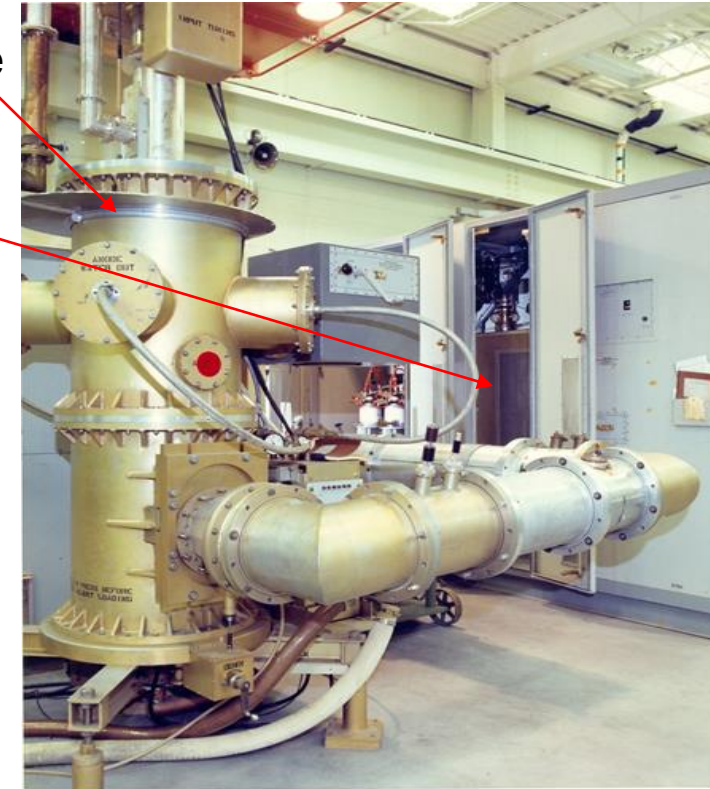
RCA 7835 Power Triode, 7 MW Peak Power
