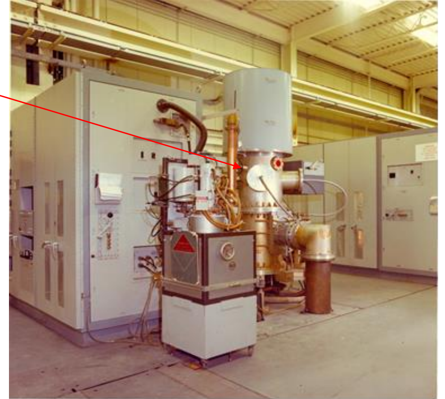
Complete RF System Driver, 5 MW PA, Modulator
