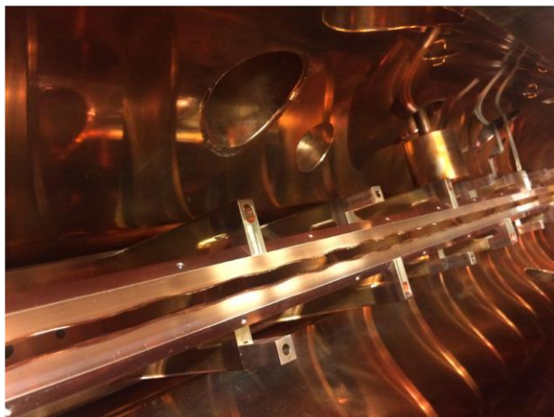
Interior of the RFQ linear accelerator*.
