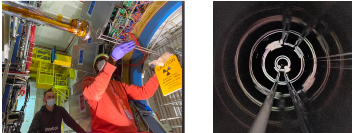
Figure 112: Left panel: Installation of the targets and holder on the East side of the STAR detector. Right Panel: A view down the beam pipe showing the three targets (C, Al, and Ni) installed at STAR.
