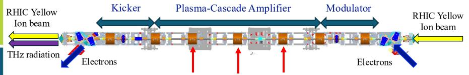
Plasma-Cascade Amplifier is a parametric amplifier: strong focusing solenoids caused periodic modulation of the beam radius and corresponding modulation of plasma frequency. It results in exponential growth of density modulation induced by ions in the modulator.
