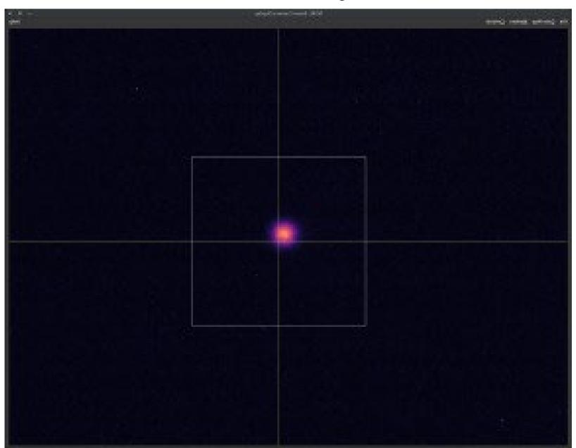
100 MeV/u deuteron beam through the dipole magnet, a 10x10cm square shown as a reference. Beam camera screen:  $\sim 130\text{cm}$  from center-of-magnet, primary beam displacement: 5 cm
