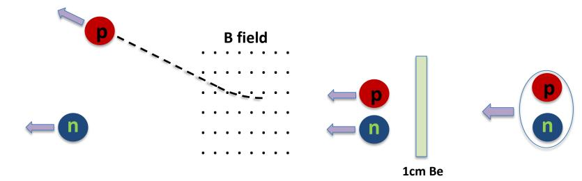
(1947) disassociation reaction strips the loosely bounded deuteron into p + n with similar energies, with a ~2% possibility for 100 MeV/n deuteron on a 1 cm Be target.
