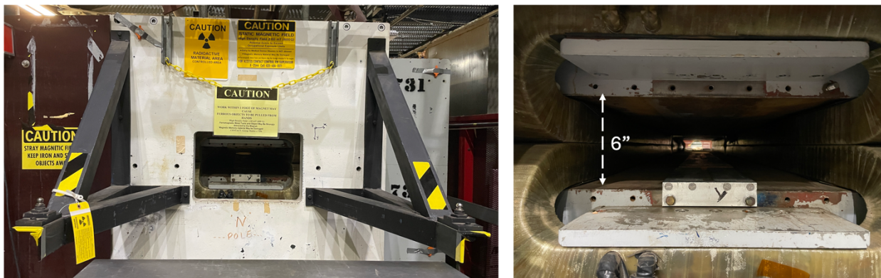
Figure 2 18D72 dipole (left) has a 6" high bore (right).
