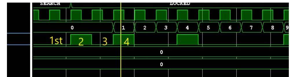
Bit\_cnt started to count when state == LOCKED
