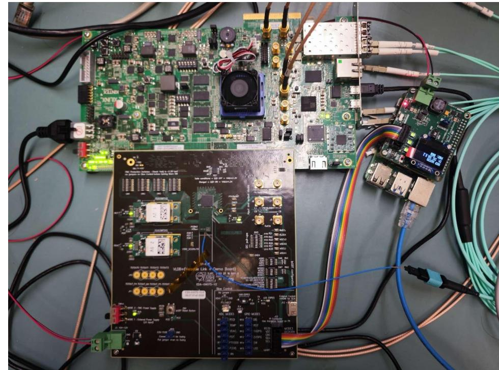
A full data path loopback test has been successfully implemented, as illustrated in the diagram. This result confirms that the initial phase (Counting Room FPGA+FCB/FIB) of our hardware test platform is operational.
