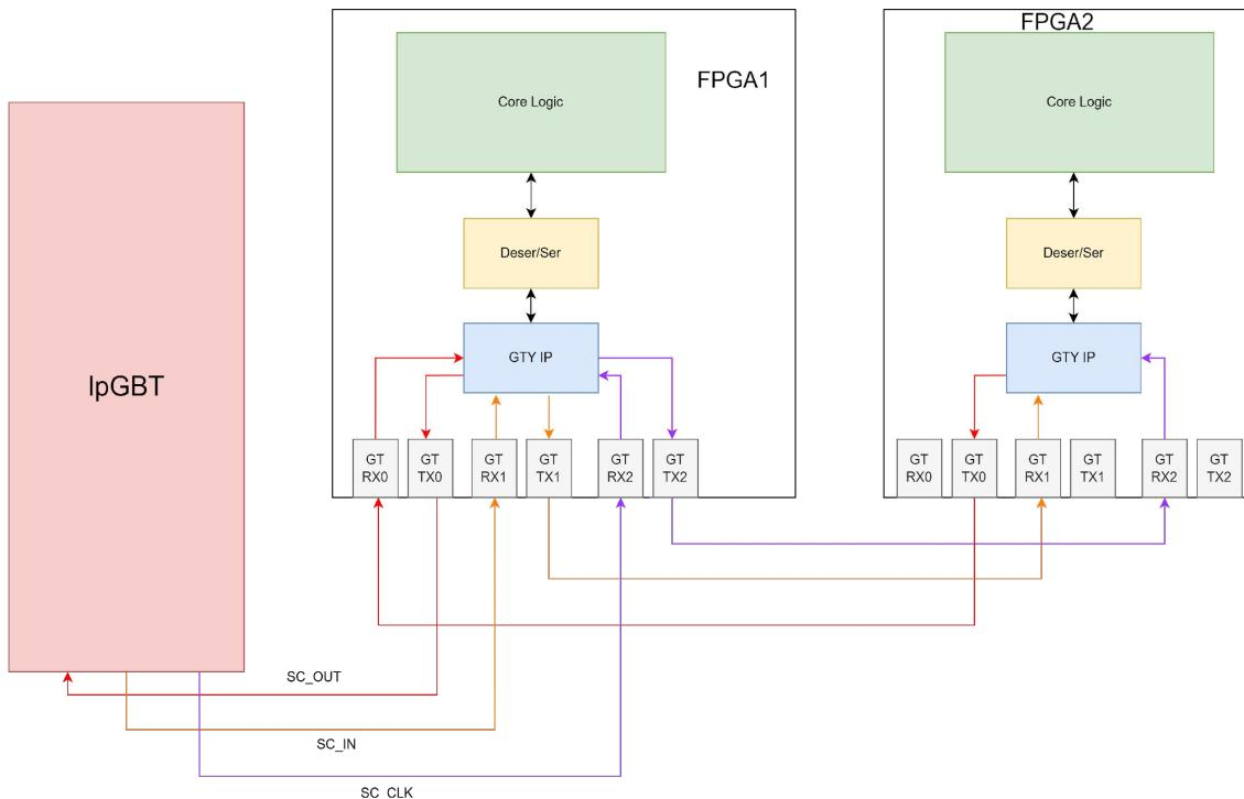
This diagram illustrates a two-AncBrain daisy-chain configuration for which the data communication link has been successfully tested and confirmed.
